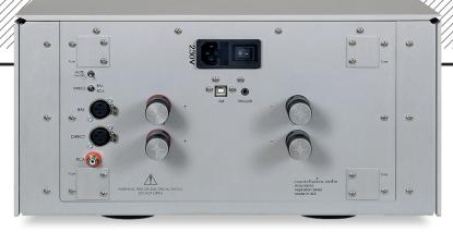
ABOVE: Constellation's Mono 1.0 has two balanced (XLR) and one single-ended (RCA) input, selected by a small toggle switch. Two sets of 'Argento Clamp' speaker cable terminals are fitted but the RS232 and USB ports are for control and updates only
